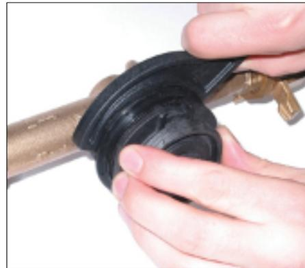
2. Replace both O-rings that are in the Flow Tube with new ones that were shipped with the FAM measuring Units. Apply a little lubricant on o-rings during this procedure.
