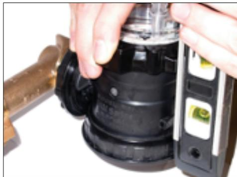
Turn locking nut clockwise to loosen.
