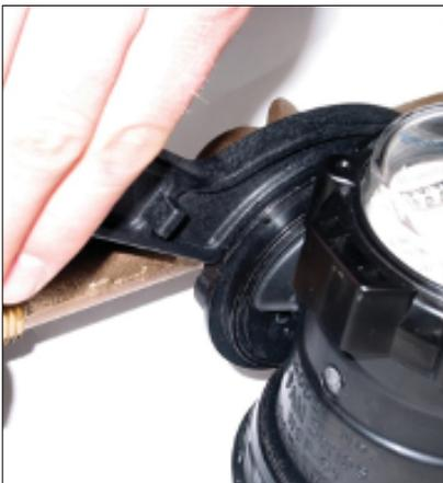
5. Tighten Locking Nut with FAM wrench until snug; do not over tighten. For leveling with level refer to F1 and F2.
